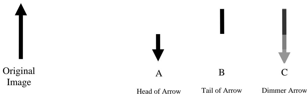
Now actually try covering half of the lens, and record the actual result on the Data Sheet and explain the result with a ray Diagram. Note that the card/paper needs to be held directly in front of the lens.
